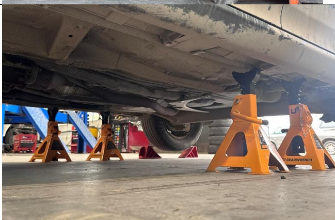
Figure 15. Overall Stability Check
