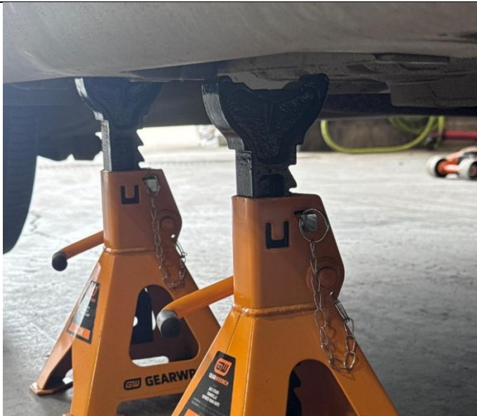
Figure 12. Primary Support Carrying Load
